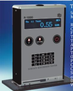
R-1000 Surface Roughness Tester Technical Data: Surface Roughness parameter Ra(ISO),Rz(DIN),Rms(Rq),Rt Ra:0.05-10.0μm/Rz:0.1-50mm Rq:0.05~10.0μm/Rt:0.1~50μm Measuring range Resolution **Cut-off lengths** Filter RC analogué 0.23in.(6mm) **Tracing length** 0.04in/second(1.0mm/second) Tracing speed ±12% of actual Value Accuracy Pick-up stylus Piezo-electric Tracer tip
