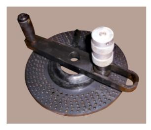
Dividing plates, crank handle sets, screws, sectors and washer are included in the accessory. There are 2 dividing plates (A and B) with hole numbers as in the table. All of dividing of 2-66, and all divisible by 2,3 and 5 from 67-132 can be carried out accurately and quickly with this accessory.
