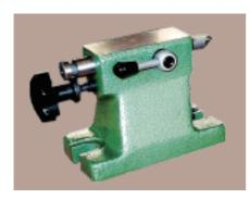
1008(WZ), 1008-0260 (TSL400-2) is designed for use with the vertical rotary tables. The tailstock is used to hold center shaft, cylinders and other workpieces for the maching of grooves, splines, flats, keyways, etc. The center is retractable for repeated operations. Center is securely locked into position with clamp. Note:Type 1008-0070(WZ70) tailstock is matched to 1003-0100(TSL100).Type 1008-0260 tailstock is matched to 1003-0400(TSL400). The tailstock for rotary table is special supplied.
