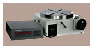
The series digital display rotary tables are for indexing.circular cutting, angle setting, boring, spot facing operations and similar work in conjunction with a milling machine. This type rotary table is so designed as to permit machining operations at a higher dimension. It can also be used for measuring exact angle.
