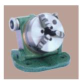
Indexing spacer perfect for small precision detail work on benchtop machines, full size mills, drills, engraving machines, jig borers, etc micro dial for easy movement of chuck 360 degree graduated ring thru hole goes all the way through indexer easy backlash adjustment tilting 0-90 degrees via graduated ring and positive lock lever.
