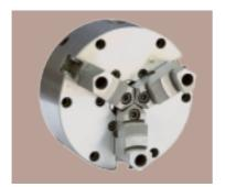
Self-centering Guaranteed To 0.0005" stock No. 1057-0008 features: Two-piece Reversible Jaws high Strength Semi-steel Body lathe Chuck Runout Adjustable To .0005" BY 3 Side screws all Jaws Are Standard Amercian Tongue Ang Groove Chuck Diameter 8..15" Thru Hole 2.48" Maximum Grip 7.30"
